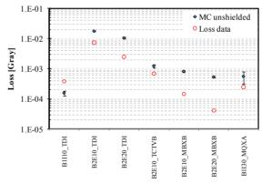
Figure 4: Comparison of FLUKA simulation and measured BLM response for beam loss on the TDI in P8.
