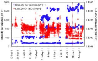
Figure 1: Normalised beamloss at TI 2 TCDI.29504 collimator in 2011. The trend is downward: the step in July coincides with stopping transverse blowup in SPS.
