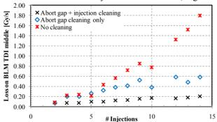
Figure 6: Injection losses at TDI with AGC and IGC.
