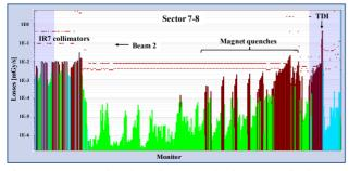
Figure 7: Losses in P8 and sector 78 after MKI flashover. 11 LHC magnets quenched with 36 bunches grazing TDI.
