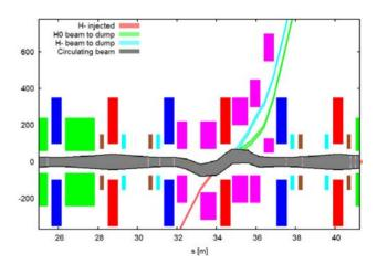
Figure 1: Layout of the H<sup>-</sup> injection system with horizontal 3  $\sigma$  beam envelopes in mm. Boxes indicate main bends (green, wide), focusing quadrupoles (red), defocusing quadrupoles (blue), horizontal and vertical painting bumpers (turquoise and brown, small) and chicane bumpers (magenta).
