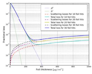
Figure 2: Optimisation of foil thickness with respect to beam losses from stripping efficiency and scattering. The optimum foil thickness is  $350 \ \mu\text{g/cm}^2$  for 10 foil hits per proton and  $320 \ \mu\text{g/cm}^2$  for 30 foil hits.
