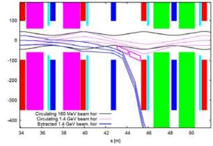
Figure 7: Extraction at 2 GeV kinetic energy from the RCS. The filled boxes in magenta and turquoise show the extraction kickers and bumpers and the magenta lines the septum blades. Beam envelopes (blue for injection energy, black for lowest extraction energy) are shown for a 3 sigma beam size including a closed orbit distortion of 1 mm.
