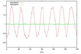
Figure 5: Beta beating for RBEND chicane and painting magnets.
