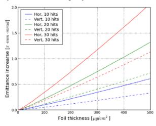
Figure 3: Emmitance increase due to multiple coulomb scattering in the foil.
