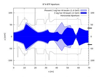
Figure 3: Horizontal 3 sigma beam envelopes for dp/p of  $1.3 \cdot 10^{-3}$ . The black bars on the right indicate the septum acceptance. The transverse emittance  $\varepsilon_x = 12 \text{ mm}$  mrad (1 $\sigma$  normalised).
