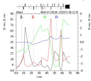
Figure 2: Transfer line optics matched in the horizontal plane to PS injection optics.
