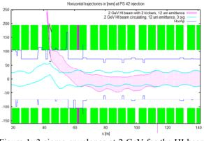
Figure 1: 3 sigma envelopes at 2 GeV for the HI beam at PS injection. The boxes in green show the PS combined function magnets, the blue line the horizontal aperture, the boxes in magenta the kicker elements in SS 45 and SS 53. The transverse emittance  $\varepsilon_x = 12 \text{ mm mrad}$  (1 $\sigma$  normalised).
