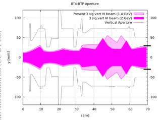
Figure 4: Vertical 3 sigma beam envelopes for dp/p of  $1.3 \cdot 10^{-3}$ . The black bars on the right indicate the septum acceptance. The transverse emittance  $\varepsilon_x = 9 \text{ mm mrad } (1\sigma \text{ normalised})$ .
