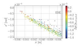
Figure 4: Phase space map (x-x') for RF-noise method of an extracted low energy proton beam at ESE with the relative momentum deviation as color code
