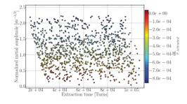
Figure 3: Correlation between initial normalized amplitude and extraction time for 400 MeV/u carbon ions with betatron core method, the extracted relative momentum deviation is color encoded
