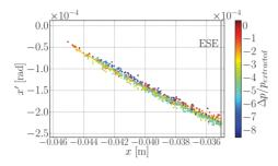
Figure 2: Phase space map (x-x') for betatron core method of extracted top energy carbon ions beam at ESE with the relative momentum deviation as color code. As expected, particles with high momentum exhibit the largest spiral step.
