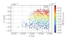
Figure 5: Phase space map (x-x') for lattice tune adjustment method of an extracted low energy proton beam at ESE with the relative momentum deviation color encoded
