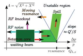
Figure 1: Steinbach diagram showing the various different driving mechanisms: a) betatron core (red), b) RF knockout (magenta), c) RF noise (cyan) and d) lattice tune adjustment (orange). The spill is indicated for case a and c.
