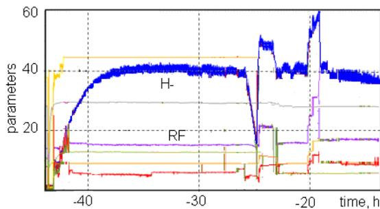
Figure 4: Evolution of H<sup>-</sup> beam intensity with variation of RF power and magnetic field.
