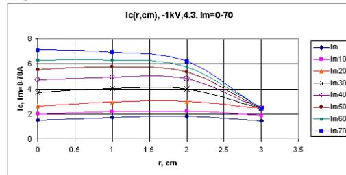
Figure 2: Radial distribution of current density of extracted positive ions for different magnetic fields (coil current  $I_m$ ), as determined from the 7 collectors.
