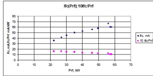
Figure 5: Evolution of the Faraday cup current  $I_{fc}$  and ratio  $I_{fc}/P_{rf}$  as function of  $P_{rf}$  during cesiation. The efficiency of  $I_{fc}$  generation increased with decreased gas flow Q from 20 sccm to 17.2 sccm.
