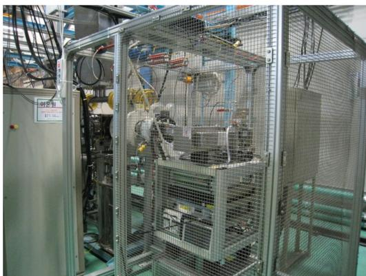
Figure 3: Microwave ion source.
