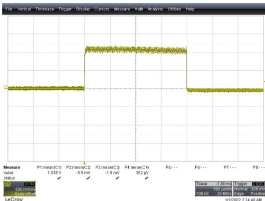
Figure 4: Pulse beam current (20mA, 2ms).
