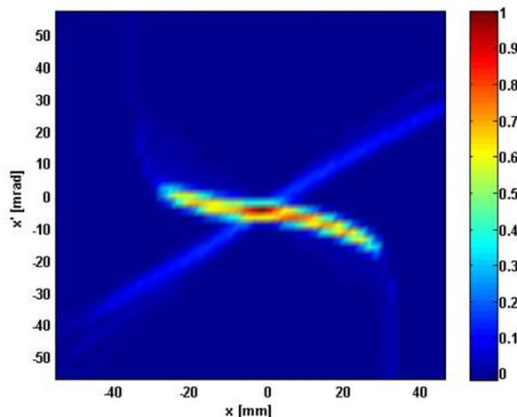
Figure 5: Beam distribution in phase space.
