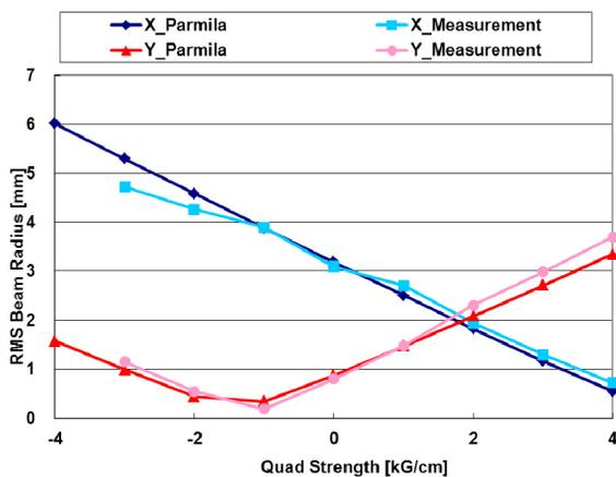
Figure 7: Comparison between beam radius measurement and simulation
