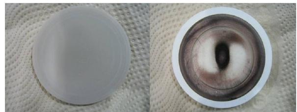
Figure 2: Microwave window after 100 hour operation test (left: Aluminum nitride, right: Boron nitride).
