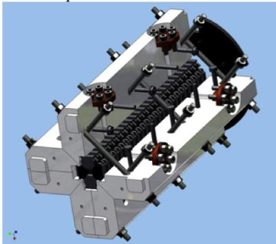
Figure 4: Cut-of the helical wiggler
