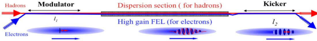
Figure 2: Economic version of coherent electron cooler, wherein electrons and hadrons are not separated transversely.
