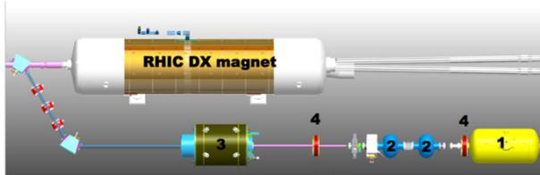
Figure 3: Layout of CeC linear accelerator: (1) 112 MHz SRF gun; (2) 500 MHz bunching cavities; (3) 5-cell BNL3 704 MHz 20 MeV SRF linac; (4) focusing solenoids.
