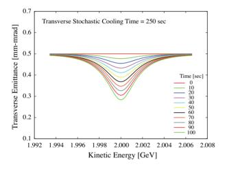
Figure 2: Transverse emittance during simultaneous use of stochastic and electron coolers for the transverse stochastic cooling time  $\tau_c = 250$  sec.
