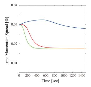
Figure 1: Momentum spread history with simultaneous use of stochastic and electron coolers. The red, green and blue curves show the results with the transverse stochastic cooling time of 250 sec and 100 sec, and without the transverse stochastic cooling ( $\tau_c = \infty$  sec), respectively.
