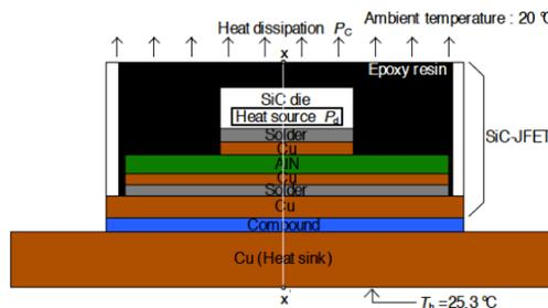
Figure 7: Thermal analysis model
