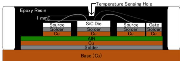
Figure 4: Cross-sectional view of the SiC-JFET
