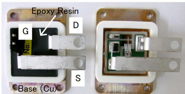
Figure 3: Appearance of the developed SiC-JFET
