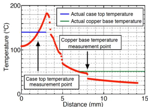
Figure 8: Temperature distribution along the centre axis of the device
