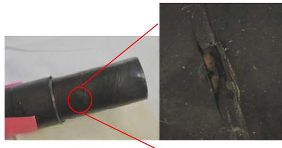
Figure 4: cable breakdown
