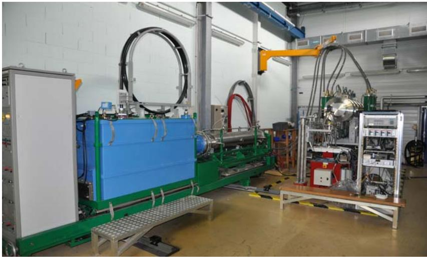
Figure 5: Test bed in use for determination of the lifetime of Airix cells and their driver.
