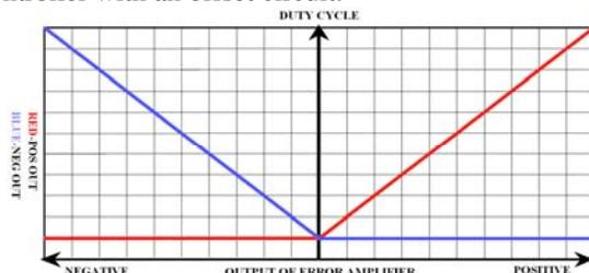
Figure 2: The relationship between the switching duty cycles and the output of error amplifier.
