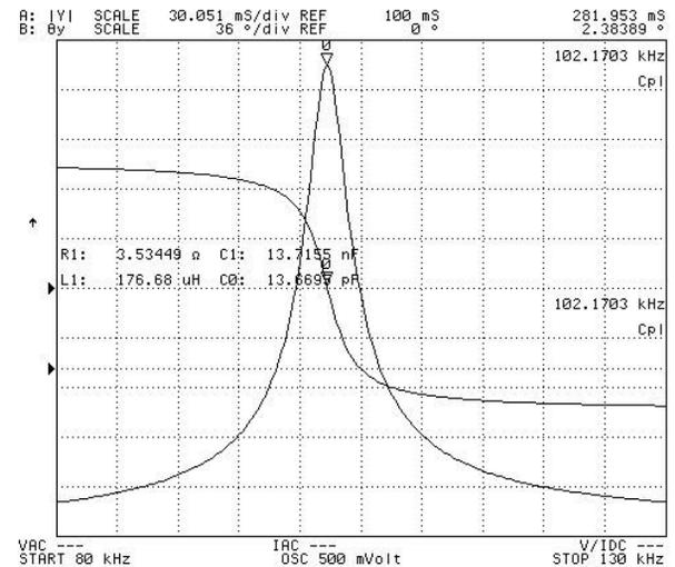
Figure 3: The diagram of scan frequency versus impedance response of the primary characteristic for the LLC resonant transformer.
