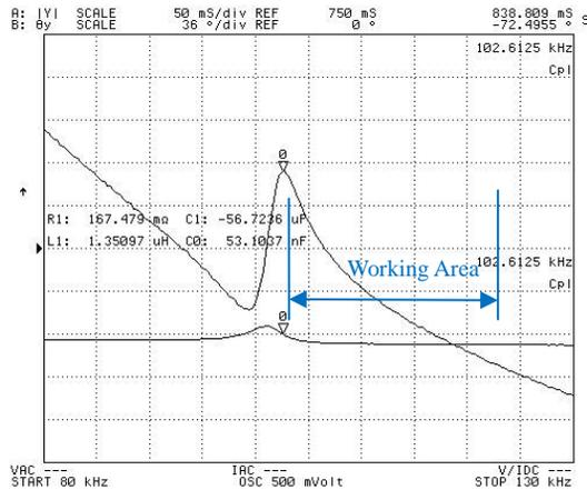
Figure 5: Impedance response diagram of the secondary characteristic for the resonant transformer.
