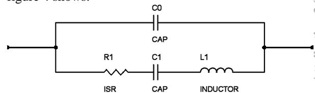
Figure 4: Type E of the Agilent 4294A LCR simulation model.
