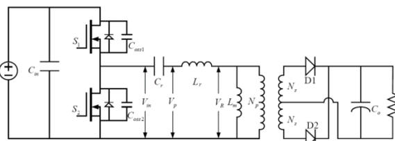
Figure 6: Resonant half bridge topology.
