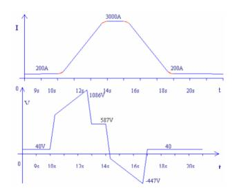
Figure 1: One kind of the current and voltage waveforms when a power supply in heavy-ion accelerator works in the pulse mode.
