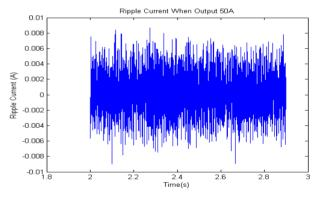
Figure 5: Ripple current.
