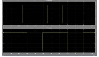
Figure 3: IGBT driving signals for positive output.
