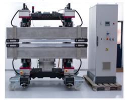
Figure 1: Finished modulator for the FEL-2 beam line, just before shipment to the FERMI@Elettra site.
