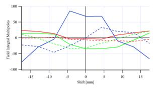
Figure 6: Shift dependent integrated field multipoles of the EPUb#2 undulator at minimum operational gap of 10 mm. All the multipoles are well within the specified limits of 100 G for quadrupoles and 100 G/cm for sextupoles. Solid lines are normal components, dashed line are skew components. Red is dipole in Gcm, green is quadrupole in G and blue sextupole in G/cm.
