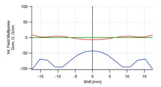
Figure 7: RADIA prediction of the shift dependent integrated filed multipoles due to the susceptibility of magnetic material in the end section. Red is dipole, green quadrupole and blue sextupole
