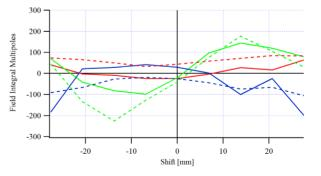
Figure 2: A measurement of the shift dependant integrated field multipoles for the EPUa#1. Measurement was done at minimum gap of 10 mm. Multipoles values drop quickly with the gap and drop down to correct values at gaps greater than 12 mm. Solid lines are normal components, dashed line are skew components. Red is dipole in Gcm, green quadrupole in G and blue sextupole in G/cm.
