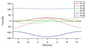
Figure 4: Magnetic forces in the vertically and horizontally polarised blocks of the EPUb. Forces shown were calculated with RADIA with a 4 period model including the susceptibility of the magnetic material.
