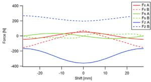
Figure 3: Analysis of the forces on a single magnet block. Forces shown were calculated with RADIA with a 4 period model including susceptibility of the magnetic material.
