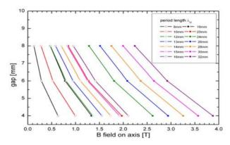
Figure 3: Gap versus K value (left plot) and gap as a function of the maximum B field on axis (right plot). Each for different period lengths.
