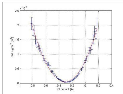
Figure 4: Typical LPM horizontal emittance measurement.
