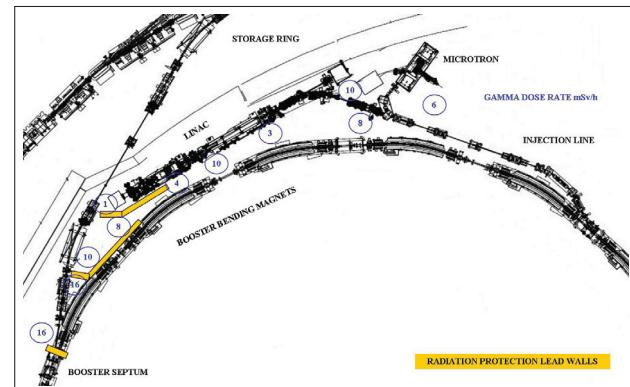
Figure 3: Radiation survey of bunker.
