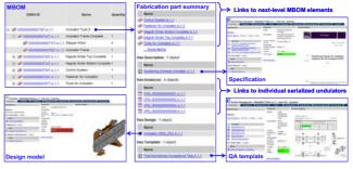
Figure 3: Sketch to illustrate information traceability in parts tracking and documentation: Seamless navigation from design model to individual physical parts and back (see text).
