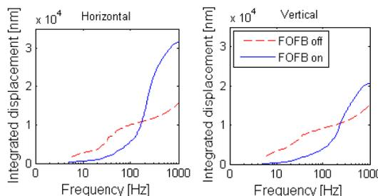
Figure 8: Integrated beam motion with and without FOFB.
