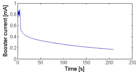
Figure 2: Decay of stored beam current.
