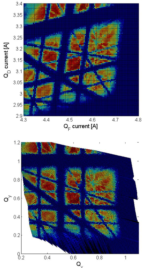
Figure 1: Integrated booster current as a function of quadrupole current (above) and betatron tune (below).
