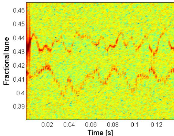
Figure 3: Stability of horizontal (upper) and vertical (lower) fractional tunes immediately following injection.
