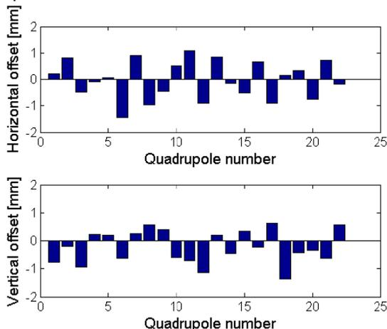
Figure 5: Results of beam-based alignment measurement.
