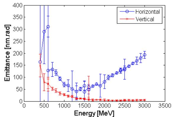
Figure 4: Transverse emittance of extracted beam.
