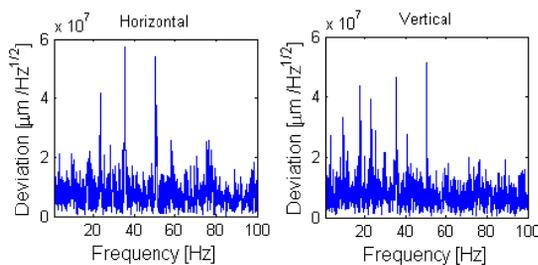
Figure 7: Noise spectrum of stored beam.
