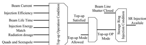
Figure 3: Top-up operation interlock logic diagram.
