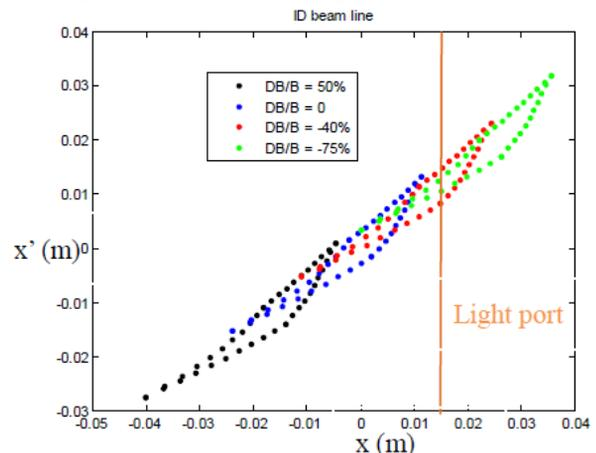
Figure 2: Track result for bend magnet short (Particles on the left side of the light port is considered as safety).
