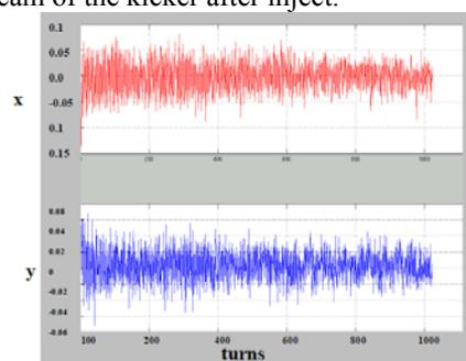
Figure 5: BPM turn-by-turn data after injection.
