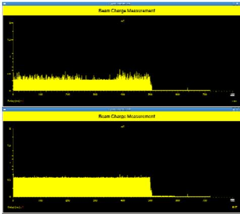
Figure 7: Bunch filling status (up, at the beginning, below, 3 hours later top-up injection).
