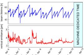
Figure 4: Typical delivery at ultra low vertical emittance (200mA with 7/8+1 filling mode). (Values during refills are not displayed).
