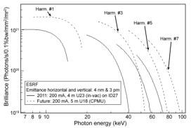
Figure 3: Brilliance of the X-ray beam emitted from the two in-vacuum undulators installed on ID27 (High Pressure beamline). Each undulator segment has a period of 23 mm, a length of 2 m and is operated with a minimum gap of 6 mm. Dashed curve: Extrapolation with two 2.5 m cryogenic in-vacuum undulators.
