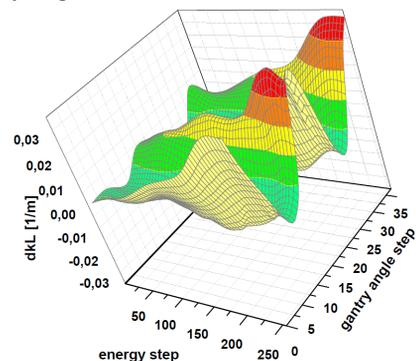
Figure 6: Correction to a quadrupole integral field gradient (dkL) as function of the gantry angle step (1 step ≡ 10°), and energy step with fit (surface) between the nodes for a fixed beam focus.
