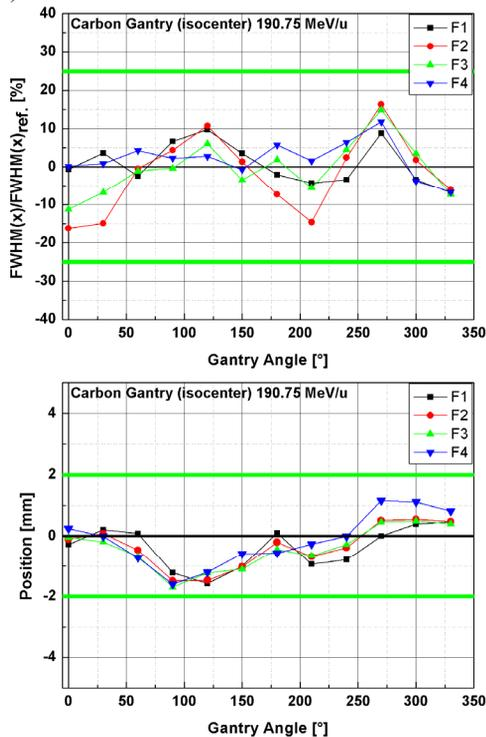
Figure 7: Carbon (190.75 MeV/u), isocenter; top: different beam widths F1-F4 (x, FWHM), relative deviation from reference values over a full gantry rotation; bottom: beam position (x) over a full gantry rotation; green lines indicate permitted limits.
