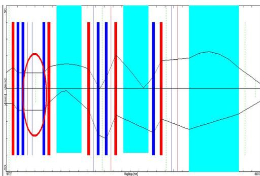
Figure 5: Beam envelopes along the gantry; red marked: envelopes at the gantry entrance point (MIRKO simulation [3]).
