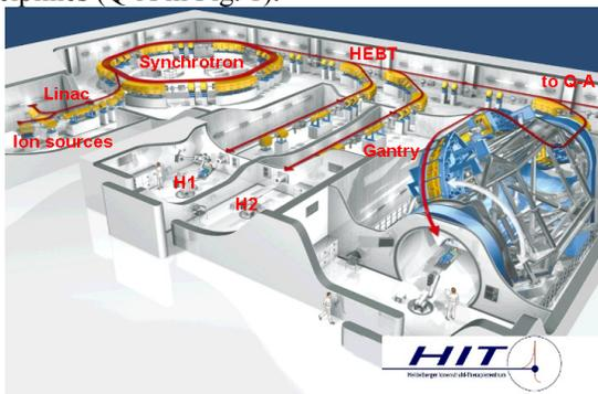
Figure 1: Overview of the HIT accelerator.
