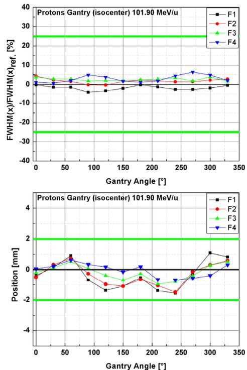
Figure 8: Protons (101.9 MeV/u), isocenter; top: different beam widths F1-F4 (x, FWHM), relative deviation from reference values over a full gantry rotation; bottom: beam position (x) over a full gantry rotation; green lines indicate permitted limits.
