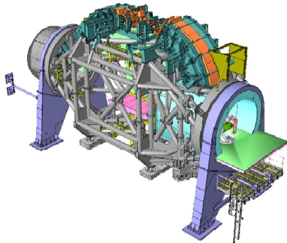
Figure 2: Drawing of the heavy ion gantry at the HIT including mechanics, beam line components and patient treatment room (MT Mechatronics).
