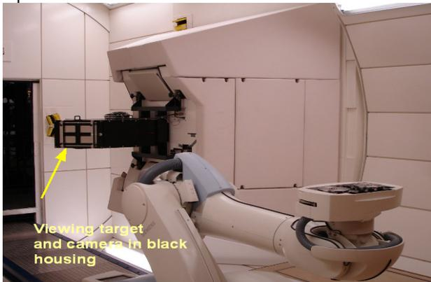
Figure 4: Viewing target and camera in black housing at the gantry nozzle (patient treatment room).
