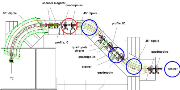
Figure 3: Gantry beam line with beam diagnostic devices (profile grid, ionization chamber (IC), not shown: scintillator, viewing screens); red circle: final focus setting quadrupoles; blue circles: final position setting dipoles/steerer.
