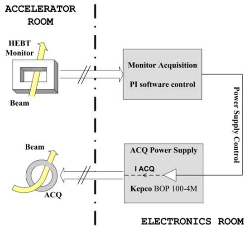
Figure 7: Servo Spill on the ACQ block diagram.
