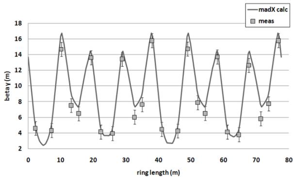
Figure 2: Absolute value of vertical beta function along the synchrotron ring at extraction.
