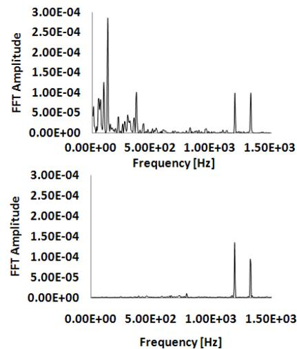
Figure 9: FFT on the QIM signal without correction on top and with correction on bottom.
