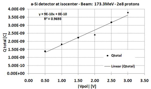
Figure 4: Detector generated total charge versus its reverse voltage.
