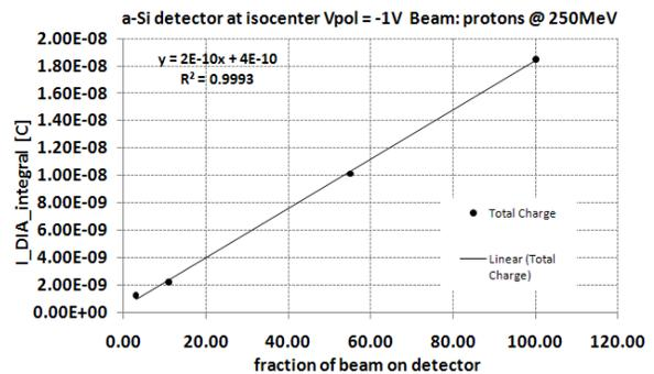
Figure 5: Total collected charge versus fraction of beam hitting the detector. 100% corresponds to  $2e9$  protons.
