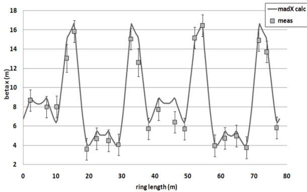
Figure 1: Absolute value of horizontal beta function along the synchrotron ring at extraction.
