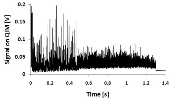
Figure 8: Intensity signal on the QIM. At  $t = 0.5s$  the servo spill loop is switched on and the intensity ripple is reduced.
