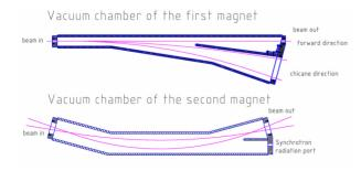
Figure 3: Technical drawing of the two chicane dipole chambers, with sketched in beam trajectories at maximum and minimum target angles.
