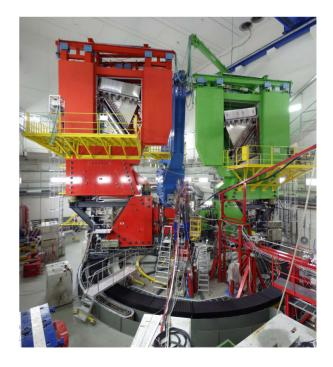
Figure 1: Photograph of the the 3-spectrometer set-up before reconstruction, spectrometers A, B and C can be seen. The beam is coming from the right.
