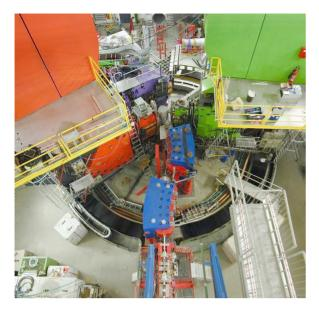
Figure 4: Photograph of the KAOS chicane inside the 3spectrometer ring (black circle: inner radius of 5.7 m). Left and right, spectrometers A and C are visible, in violet the KAOS dipole can be seen. The small blue magnets are the former DCI bending magnets. The flange of beam dump is located in the top middle of the picture.
