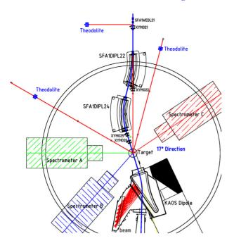
Figure 2: Overview over the KAOS chicane and the theodolite positions for target adjustment. The beam is coming from the top of the picture and is going to the bottom, following the blue line  $(17^{\circ} \text{ target angle})$ .
