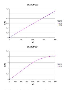
Figure 5: Plots of the B-fields of the chicane magnets as a function of current I.
