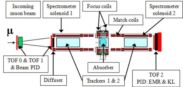
Figure 1: Step IV configuration of the MICE Experiment.
