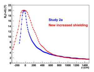
Figure 4: Comparison of the  $B_z$  magnetic field profile along the z axis for the Study 2a (blue squares) and the increased shielding (red circles) geometries.
