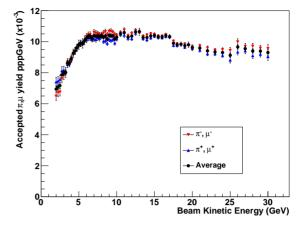
Figure 6: Close-up of the distribution of the accepted pion and muon yields (per proton per GeV) for the new increased shielding target geometry for proton beam kinetic energies between 2 and 30 GeV.
