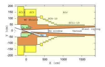
Figure 3: Schematic of the target station geometry with increased shielding to protect the superconducting coils (SC) from high radiation doses.
