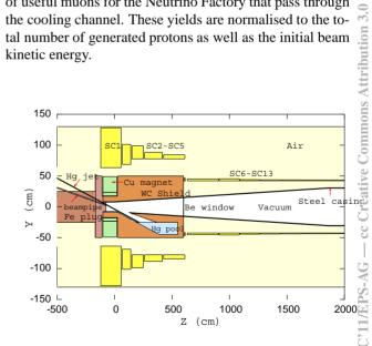
Figure 1: Schematic of the Study 2a target station geometry for the Neutrino Factory. The superconducting magnets are labelled SCn, where n = 1 to 13. The shielding consists of 80% tungsten-carbide and 20% water.
