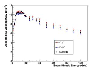
Figure 5: The accepted pion and muon yields (per proton per GeV) for the new increased shielding target geometry for a wide range of proton beam kinetic energies between 2 and 100 GeV.
