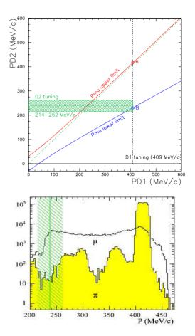
Figure 2: Top: kinematic limits for muons provided by pion decays. The red and the blue lines are the upper and the lower limits of the muon spectrum as a function of the momentum selected by the first dipole. Bottom: simulation of the muon and pion spectra at the exit of the decay solenoid. Only high momentum pions survive. The green band shows the acceptance of D2, when tuned for backward-going muons.
