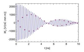
Figure 2: Long-range dipole wake of SLAC linac structure over two time ranges, with the bucket locations indicated by the red dots (lower figure).
