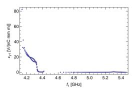
Figure 1: Dipole mode frequencies and kick factors for the SLAC structure, as obtained by the two-band circuit model.
