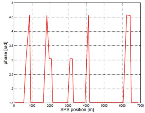
Figure 2: Phase advance in radians between SPS vertical BPMs.
