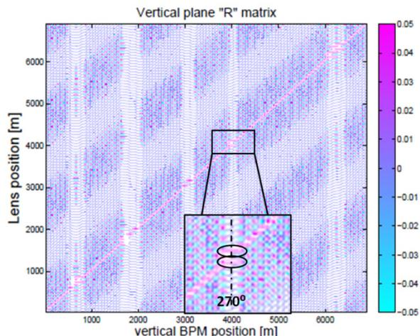
Figure 3: Vertical plane response matrix color coded with maximum response.
