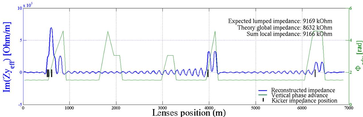
Figure 4: Vertical reconstruction of kicker impedances. Black lines are where the 19 kicker impedances are placed, green line is the vertical phase advance between consecutive BPMs in SPS, blue line is the reconstructed position of impedances.
