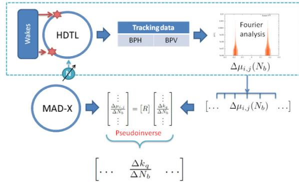
Figure 1: Scheme of the simulation set up using the HEADTAIL code.
