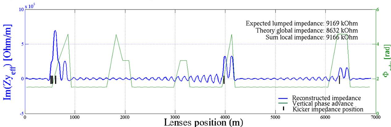
Figure 4: Vertical reconstruction of kicker impedances. Black lines are where the 19 kicker impedances are placed, green line is the vertical phase advance between consecutive BPMs in SPS, blue line is the reconstructed position of impedances.
