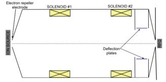
Figure 2: Schematic layout of the LEBT with the chopping system located after the second solenoid.
