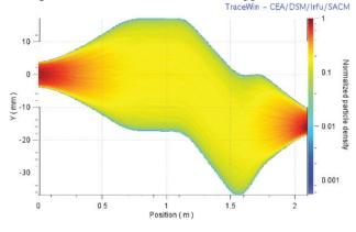
Figure 4: Beam distribution with chopper between solenoids.
