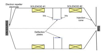
Figure 1: Schematic layout of the LEBT with the chopping system located between solenoids.
