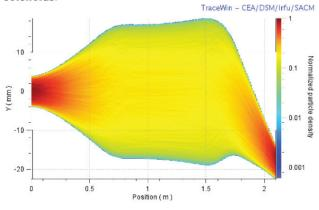
Figure 5: Beam distribution with chopper after the second solenoid.
