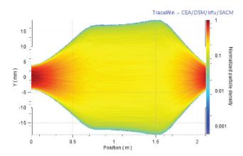
Figure 3: Beam distribution with chopper turned off.
