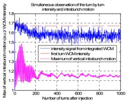
Figure 4: Simultaneous measurements of losses at injection with the WCM (blue) and the maximum of the directional coupler BPW intrabunch vertical motion (magenta). The losses occur when the vertical motion reaches its maximum, indicating a fast transverse instability.
