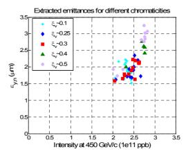
Figure 6: Vertical emittance at SPS extraction (norm. 1σ) and overall losses as a function of extracted intensity with a long SPS cycle and impact of vertical chromaticity.
