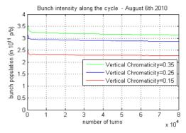
Figure 2: SPS BCT intensity data as a function of vertical chromaticity. The extracted PS intensity was between 3.4 and 3.6e11 p/b in the three displayed cycles.
