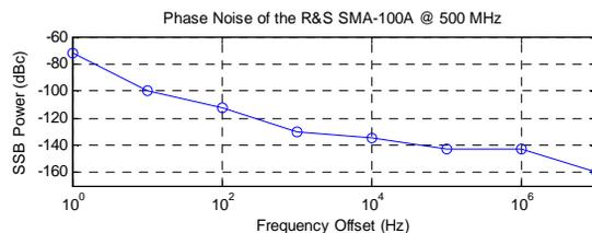
Figure 1: Nominal phase noise in dBc (1 Hz) of the R&S SMA-100A signal generator with SMA-B22 option.
