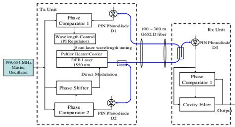
Figure 3: Simple block diagram of the Libera Sync fiber link for 500 MHz operation.
