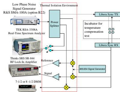
Figure 6: Functionality and performance test set up for Libera Sync pairs by using instruments in hand.
