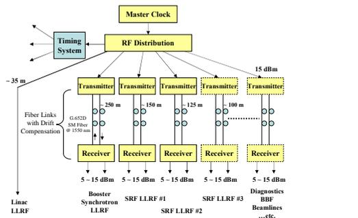
Figure 4: RF reference distribution scheme for the TPS.
