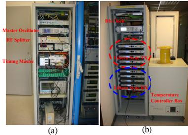
Figure 5: (a) Prototype master oscillator and the timing master. (b) Photo of the Libera Sync pairs in testing.
