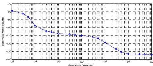
Figure 8: Measured SSB phase noise from 10 Hz to 10 MHz.
