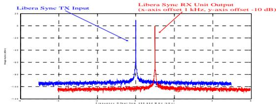
Figure 7: RF signal spectrum of Libera Sync pair input and output.
