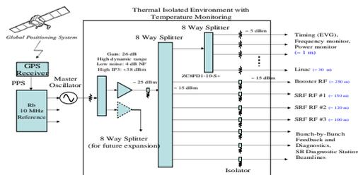
Figure 2: RF reference fanout unit.
