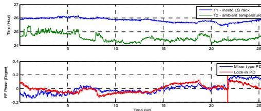
Figure 9: Preliminary long-term drift measurement results. The phase drift is most likely contributed by the phase detector which is installed at a rack without thermal isolation.
