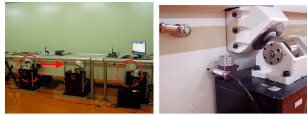
Figure 6: Contact sensors at side of girders.
