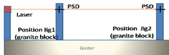
Figure 2: The architecture of laser positioning.
