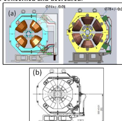
Figure 6: (a) Pole boundary diameters of quadrupole and sextupole magnets are 74mm and 78mm respectively (b) The dimension diagram of the quadrupole magnet.
