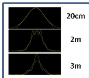
Figure 4: The beam distribution from 20cm to 3m.
