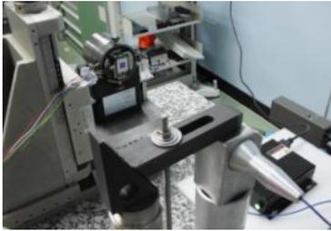
Figure 8: The arrangement of stability test of circular PSD module.
