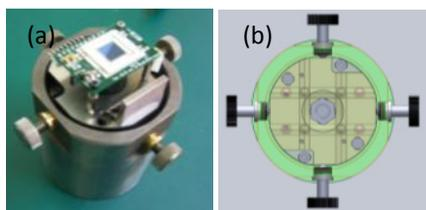
Figure 5: (a) The picture of the PSD circular steel module (b) Horizontal and vertical directions is guided by steel balls and v-cut tracks.
