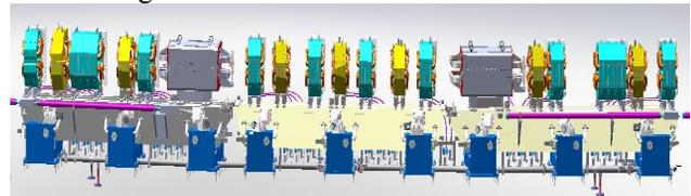
Figure 1: The arrangement of 1-cell DBA lattice magnets on three girders.
