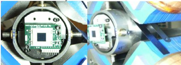
Figure 9: The PSD circular module is installed in quadrupole magnet. The gap between the PSD module and pole of magnet are over 50 $\mu$ m.
