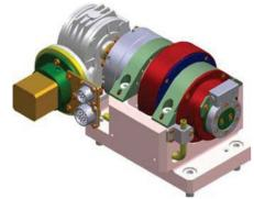
Figure 4: 3D model of cam mover.
