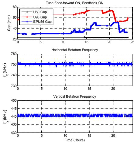
Figure 7: Tune keeps constant when feedback loop is closed.
