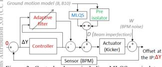
Figure 3: Control scheme including MLQS, preisolator and IPFB.
