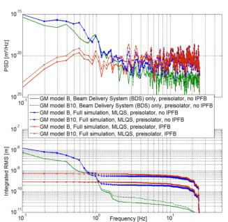
Figure 4: PSD and integrated RMS of the offset between the beams at the IP for different ground motion and configuration.
