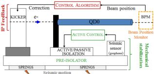
Figure 1: Overall layout of the FF stabilization.
