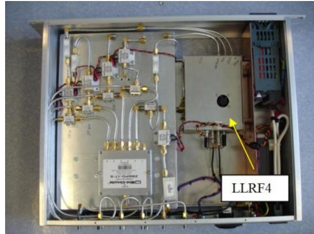
Figure 1: The LLRF4 Development Board
