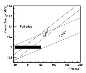
Figure 2: Acceleration scheme in simulation study. Bucket area regions are plotted by surrounding lines, and black square shows injected beam.
