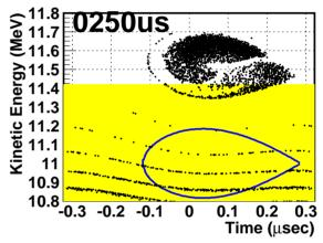
Figure 6: Phase distribution at  $t=250 \ \mu s$ .
