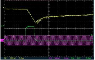
Figure 1: Bunch monitor signal during acceleration up to 100 MeV (CH1, yellow). CH3 (pink) shows rf source signal and CH4 (green) gate signal of beam chopper at ion source: 5  $\mu$ s/div.
