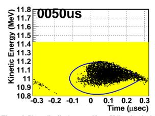
Figure 5: Phase distribution at  $t=50 \ \mu s$ . Yellow hatched region shows the energy at which closed orbit hits the stripping foil.
