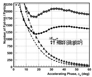
Figure 4: Averaged Number of foil hit per particle  $(N_{hit})$ . Circles are for all particles, while lost particles are neglected in triangle markers.
