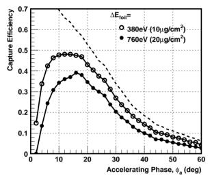
Figure 3: Capture efficiencies as functions of accelerating rf phase for different energy losses at stripping foil. Dashed line shows the result without energy loss.
