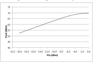
Figure 6: Gain response of the SSPA
