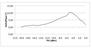
Figure 8: Phase deviation of the SSPA
