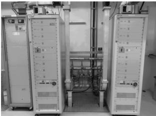
Figure 4: 10 kW SSPA (BRUKER) Two SSPA at ELBE, left rack: 10kW klystron amplifier
