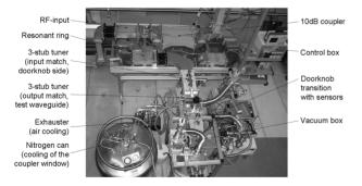
Figure 1: Layout of the resonant ring
