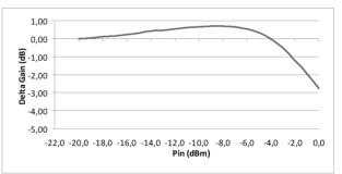
Figure 7: Gain deviation of the SSPA
