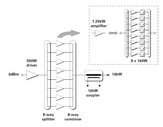
Figure 5: Block diagram of the RF-part
