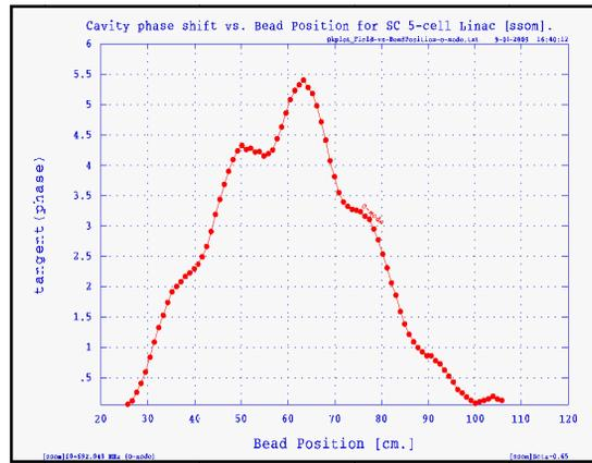
Figure 5: Plot of  $\tan \phi (\alpha |E|^2)$  vs. Bead position (for 0-mode).
