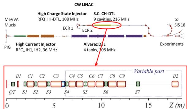
Figure 1: Future layout of the new sc cw LINAC in parallel to the existing GSI UNILAC (Ci = Cavity, Bi = (Re-)Buncher, Si = Solenoid, QT = Quadrupole-Triplet).
