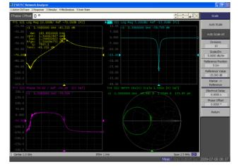
Figure 4: EMMA RF cavity response using VNA showing notch in response.
