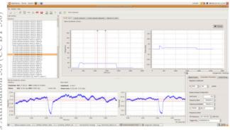
Figure 6: Beamloading signal showing power being drawn from a cavity.
