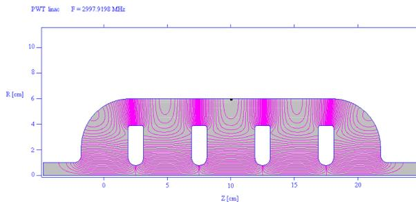
Figure 2: E-field distribution inside the PWT structure; calculated by SUPERFISH.
