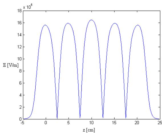
Figure 3: Accelerating field magnitude on the beam axis of the PWT structure; calculated by SUPERFISH.
