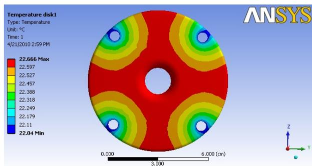
Figure 5: Steady state temperature distribution on the surface of disks for 22°C coolant water.
