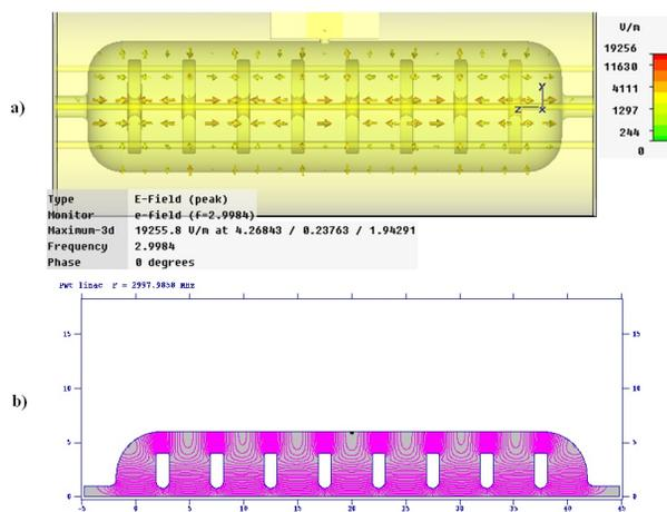
Figure 6: E-field distribution inside the PWT structure; calculated by a) CST Microwave Studio and b) SUPERFISH.
