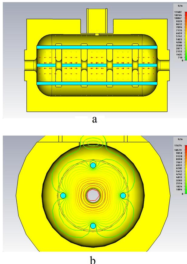
Figure 4: a) E-field arrays inside the PWT structure and b) E-field contours in transverse cross section view.
