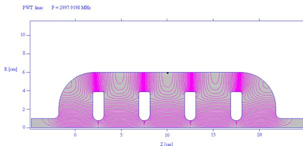
Figure 2: E-field distribution inside the PWT structure; calculated by SUPERFISH.
