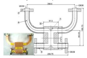
Figure 7: X-band hybrid H-plane
