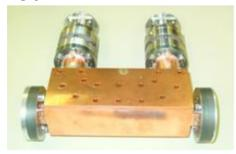
Figure 3: Bi-directional coupler by GYCOM Ltd
