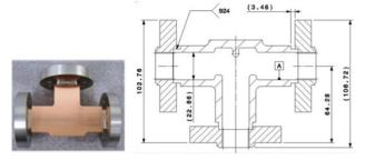
Figure 6: X-band splitter
