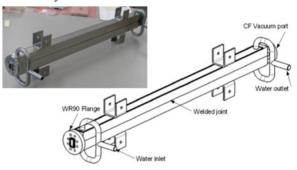
Figure 1: 3D model of X-band high power load
