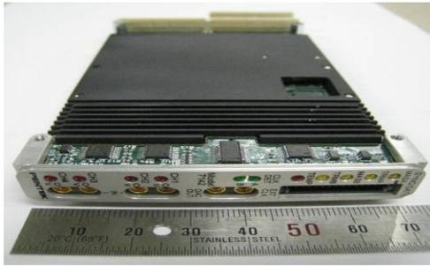
Figure 5: New commercial FPGA board (Pentek 7142).
