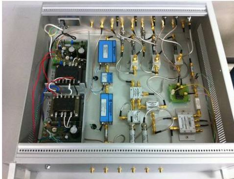
Figure 6: LLRF analogue chassis.
