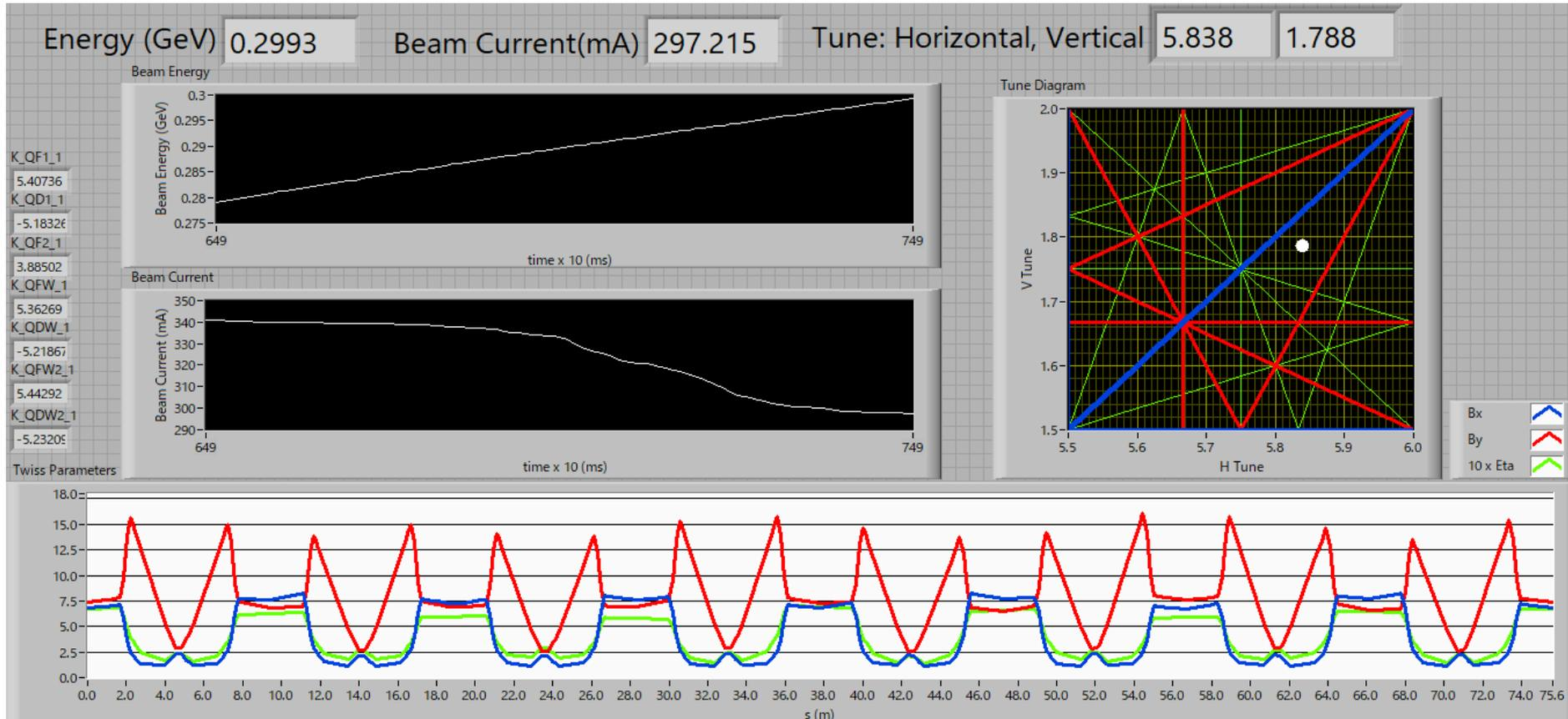
GUI for calculation of the tune and twiss parameters.
