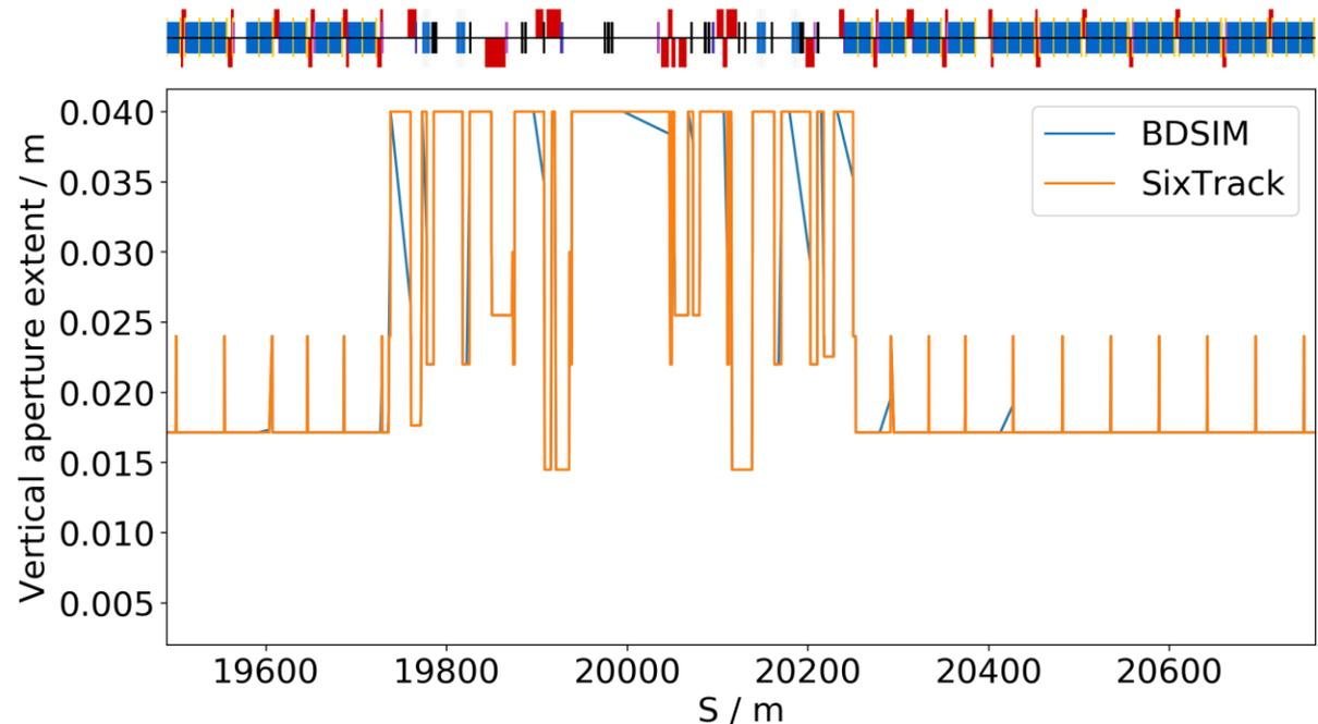
BDSIM and Sixtrack aperture models compared. Vertical aperture extents.
