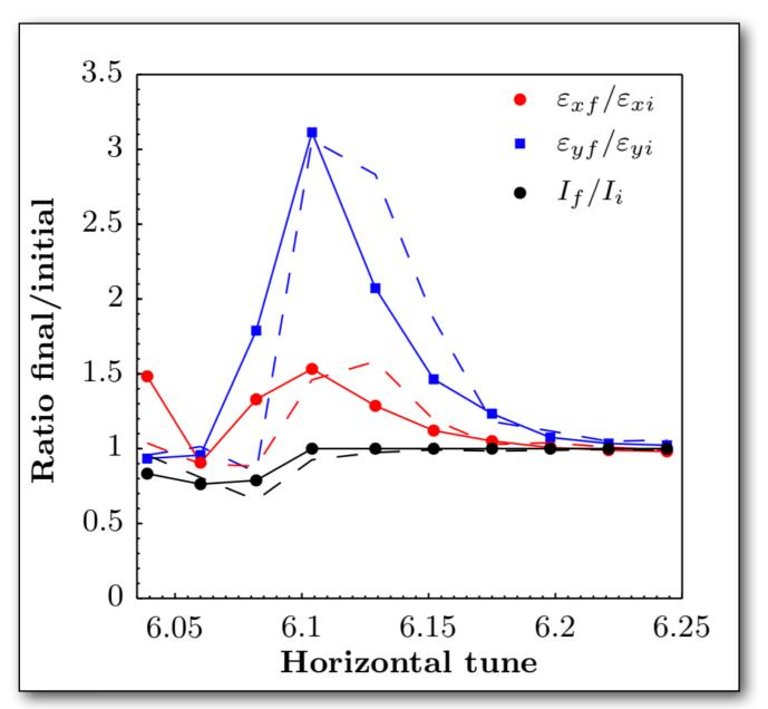
Emittance growth and beam intensity as computed with MAD-X (adaptive mode). Experimental data are shown with dashed lines.
