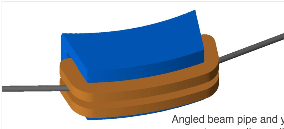
Angled beam pipe and yoke geometry as well as coils
