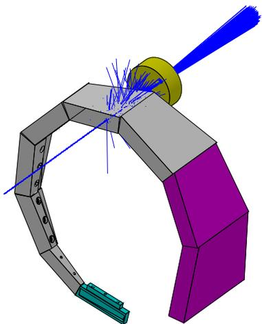
Based on realistic geometry of the IBA "wheel" degrader
